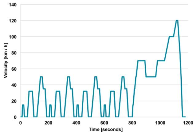
**Figure 5:** The NEDC drive cycle
